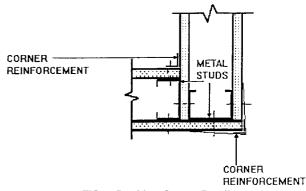
FIG. 2 Partition Corner Detail
