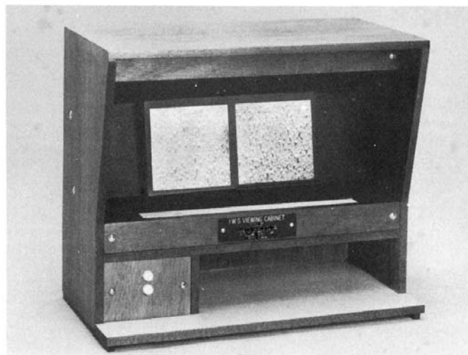
FIG. 2 Apparatus for Fabric Evaluation
