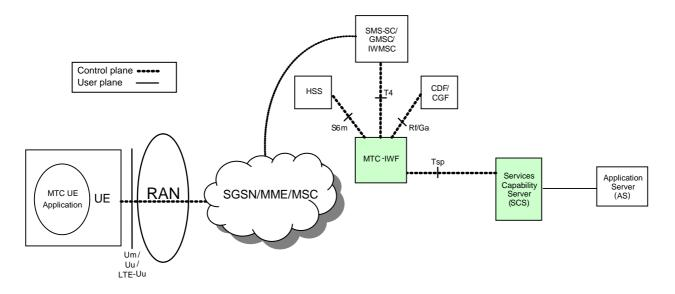
Figure 4.1.1: Tsp reference point at 3GPP Architecture for Machine -Type Communication
