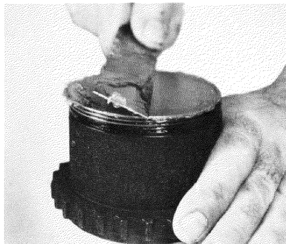
FIG. 2 Preparing Sample for Penetration Measurement
