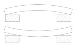
Figure 2 — Possible cause of oscillation of beams on supports
