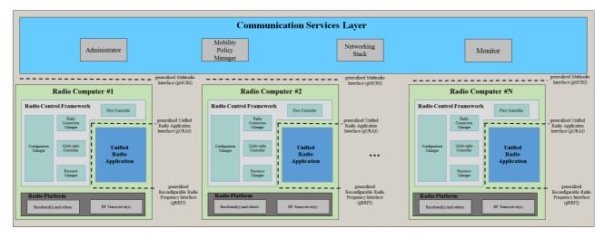
NOTE: Interfaces gMURI, gURAI and gRRFI in Figure 4.2.1-1 are used to interconnect components of different stakeholders.
