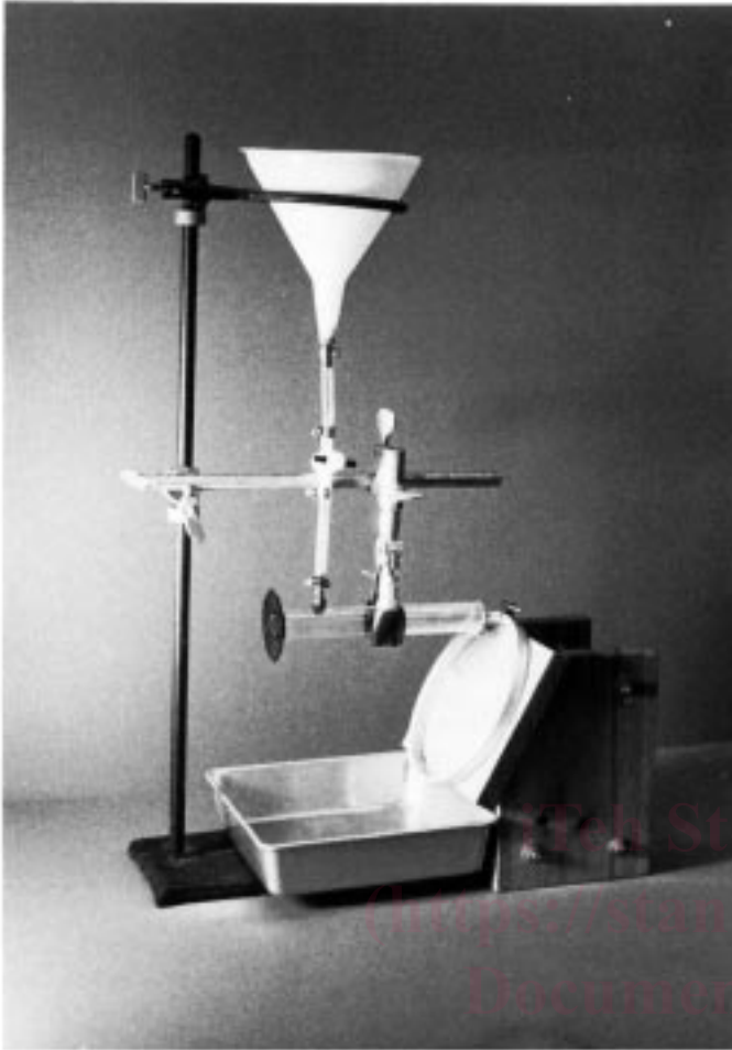
FIG. 2 A Typical Water Flow Tester
