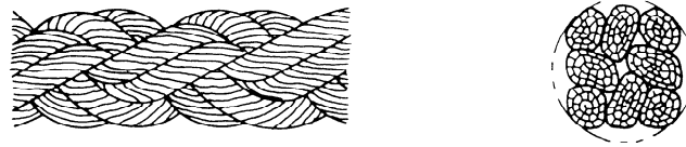
Figure 3 — Shape of an 8-strand square-plaited rope (type E)
