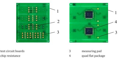
Figure 2 — Example of the position of components
