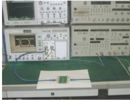
Figure 10 — Example of set-up for measurement of eye patterns
