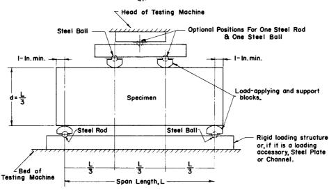
Note 1—This apparatus may be used inverted. If the testing machine applies force through a spherically seated head, the center pivot may be omitted, provided one load-applying block pivots on a rod and the other on a ball.
