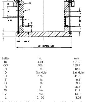
FIG. 1 Mold with Ring for Compaction of Specimen for Expansion Index Test
