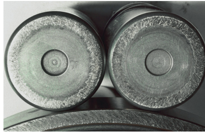
Figure 13 — Smearing on the side face of rollers of a cylindrical roller bearing
