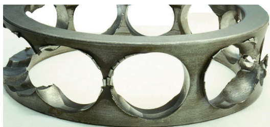
iTeh STANDARD PREVIEW Figure 9 — Advanced abrasive wear on the cage pockets of a solid metal cage (standards.itih.ai)
