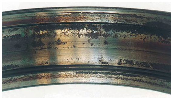
Figure 15 — Moisture corrosion on the outer ring raceway of a cylindrical roller bearing
