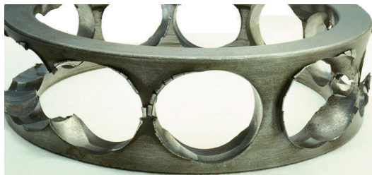
Figure 9 — Advanced abrasive wear on the cage pockets of a solid metal cage
