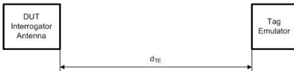
Figure 2 — Interrogator demodulation and turn around test setup
