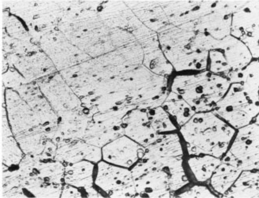
FIG. 3 Acceptable Structure Practice W—Oxalic Acid Etch Test Dual Structure Some Ditches But No Single Grain Completely Surrounded
