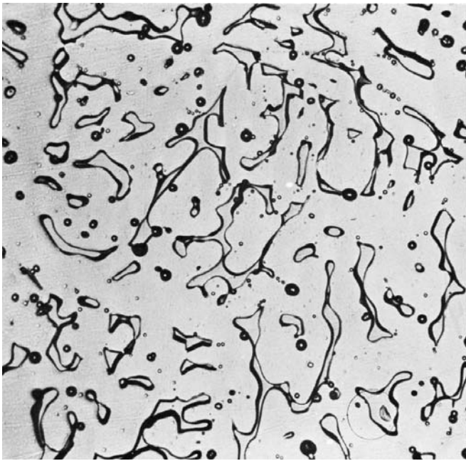
FIG. 4 Isolated Ferrite Pools (250×) (Observed in castings and welds. Steps between austenite matrix and ferrite pools)
