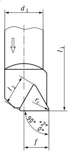
This figure shows a right-hand tool holder (R); left hand tool holder (L) laterally reversed. NOTE
