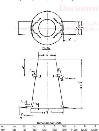
FIG. 1 Mold for Slump Test
