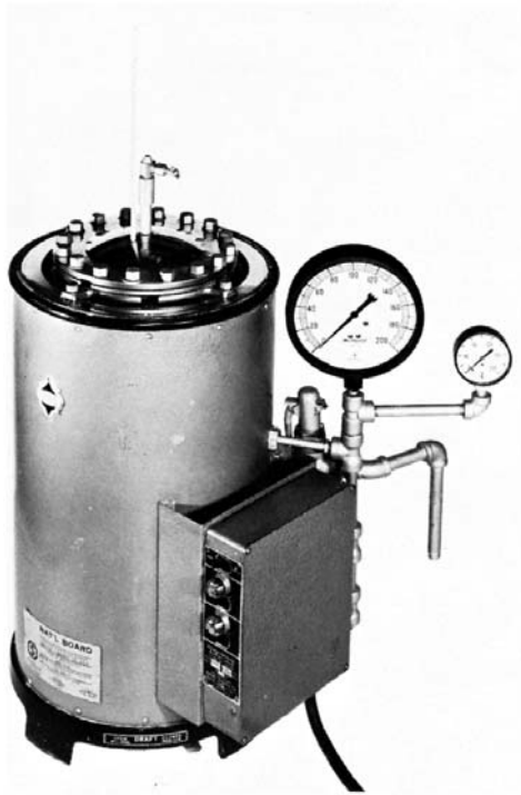
FIG. 1 Suitable Apparatus for Measuring Hydration Resistance of Basic Brick and Shapes (See 1 )
