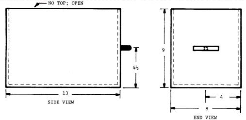
NOTE 1—Material specified is type 316 stainless steel (S.S.) or other suitable alloy (1/4 in. (6 mm) recommended). NOTE 2—All dimensions minimum outside diameter.
