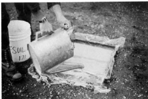
FIG. 4 Sand Being Poured Into the Template
