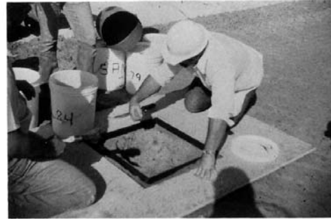
FIG. 5 Excavation of the Test Pit
