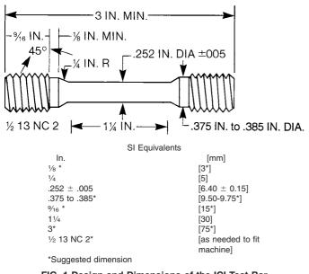
FIG. 1 Design and Dimensions of the ICI Test Bar
