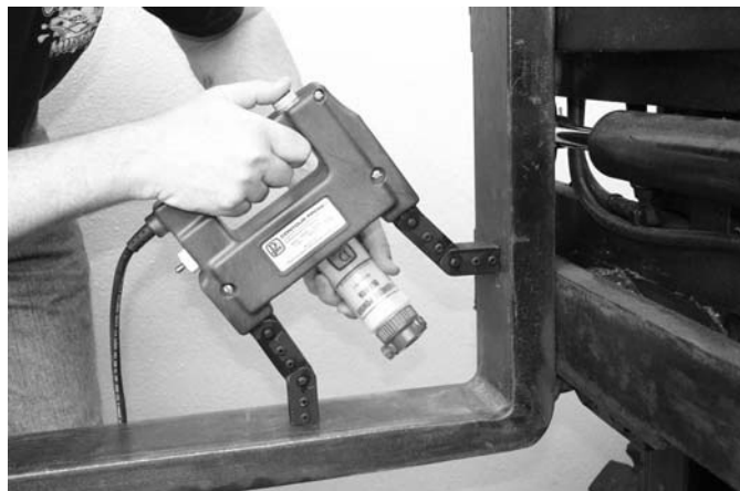
FIG. 1 Yoke Method of Part Magnetization
