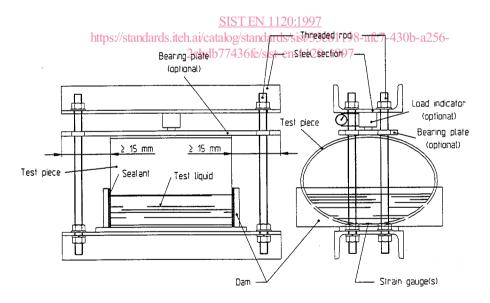
Figure 1: Typical test arrangement
