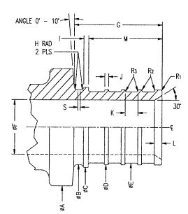
Note 1—All dimensions shall be measured with appropriate micrometers, such as pin or ball micrometers for wall thickness, and outside-diameter micrometers with flat anvils, or vernier calipers, to measure outside diameter and width of cold-expansion fittings and compression-sleeves. Note 2—The average measurement is obtained from measurements taken in at least four locations spaced at approximately 45° around the circumference, in accordance with 10.1.
