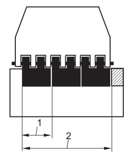
b) Width of fastening equal to the pitch times three
