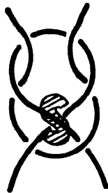
FIGURE 4 – Weaver's knot – S-type
