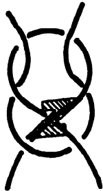
FIGURE 3 – Weaver's knot – Z-type
