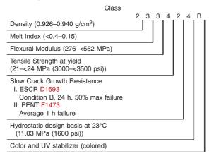
4.2 Materials used in polyethylene plastic pipe and fittings shall use a cell-type format for the identification, close characterization, and specification of material properties. The information from the format is to be used alone or in combination.
