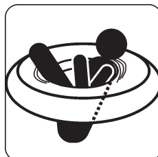
Figure 2 — Risk of getting entrapped if size is not appropriate
