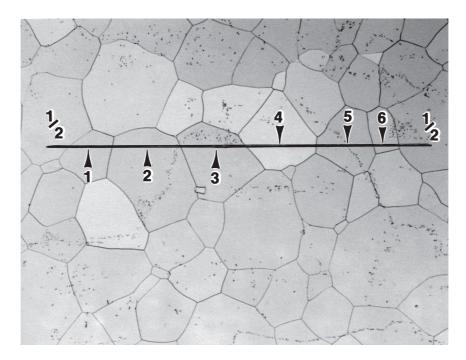
Interception, *N*, counts for a straight line on a single-phase grain structure where the arrows point to 6 intercepts and two line segments ending within grain  $(2 \times 1/2 = 1 N)$  and N = 7
