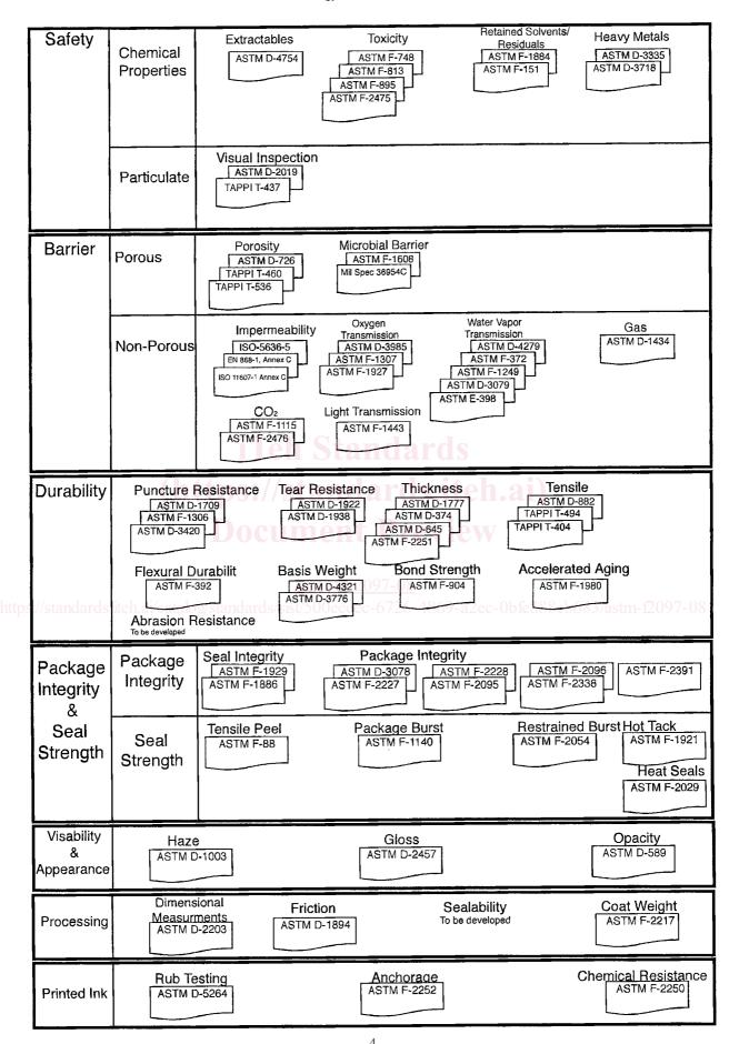
FIG. 1 Summary of Test Methods for Medical Packaging Design and Evaluation
