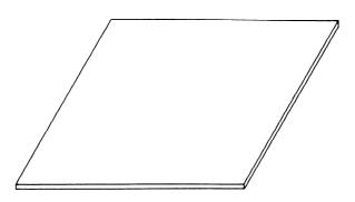
1a Flat plate, 1,5 mm thick, of stainless steel or nickel-plated steel polished on the lower surface
