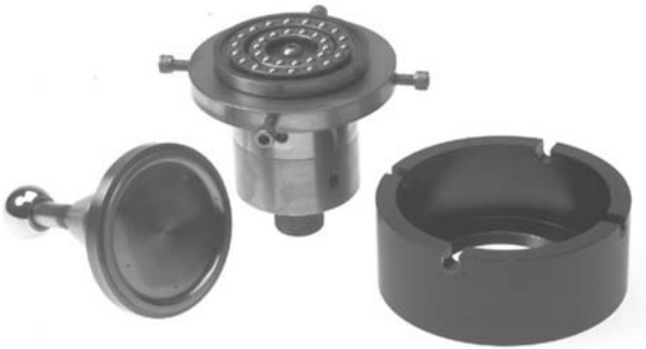
FIG. 1 Representative Unconstrained Planar Bearing Fixture for Femoral Component
