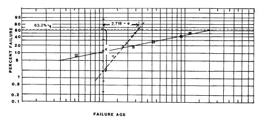
Note 1—Plotting percentage are 100 times the average of  $(n - \frac{1}{2})/N$  and n/(N + 1). Artificial data were placed on a line (dashed) drawn to illustrate a Weibull line with a  $\beta$  of 4. A second line (not dashed) illustrates the distribution of failure times which are characteristic of materials with very flat volt-time curves, such as mica composites. This line has a  $\beta$  value of 0.7.
