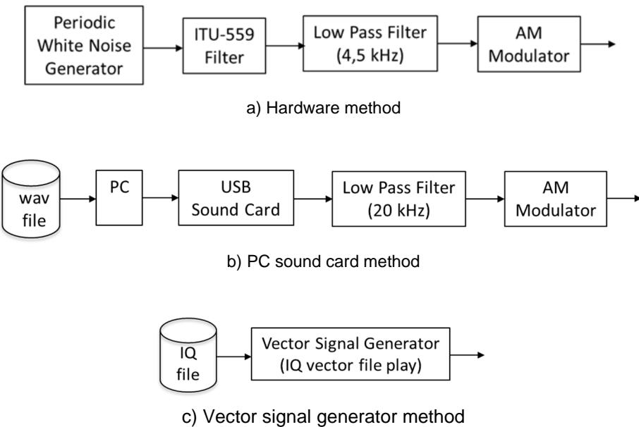
NOTE: In a), the low pass filter has a cut-off frequency of 4,5 kHz and a minimum roll-off of 60 dB/octave; in b), the low pass filter has a cut-off frequency of 20 kHz and a minimum roll-off of 40 dB/octave.
