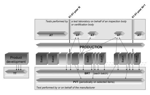
Figure 2 — Typical scheme for the assessment of conformity by a manufacturer, including a third party certification
