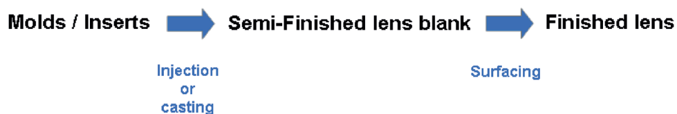
Figure 2 — General lens manufacturing flow with semi-finished lens blanks and surfacing
