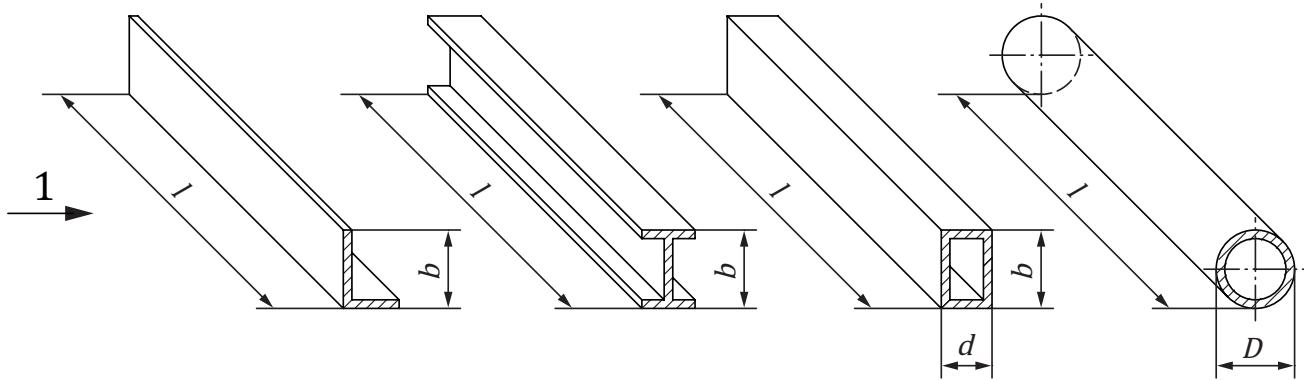
$$\text{Aerodynamic slenderness length of member} = \frac{\text{length of member}}{\text{breadth of section across wind front}} = \frac{l}{b} \text{ or } \frac{l}{D}$$
