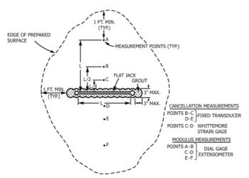
FIG. 1 Recommended Flatjack Measurement Array, Surface Measurements
