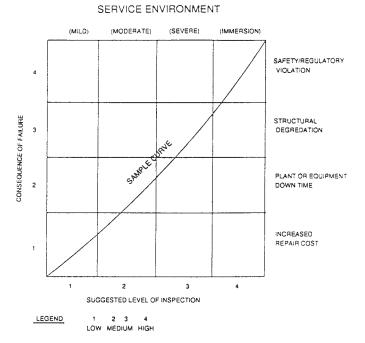
NOTE 1—This figure is provided as a visual aid to represent graphically the general relationship between the consequence of failure and the suggested level of inspection. The slope and configuration of the curve will vary due to the many factors affecting the consequence of failure, however, the suggested level of inspection should increase when the service environment is more severe.
