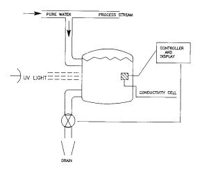
Note 1—The unit employs available water system pressure to rinse the line and test chamber, followed by a downstream valve closure that isolates the sample. Subsequent irradiation with intense UV light breaks down organic compounds in the water, with the liberated carbon forming carbon dioxide in solution as carbonic acid. By monitoring the change in sample conductivity, corrected for temperature, the TOC concentration is calculated and displayed.
