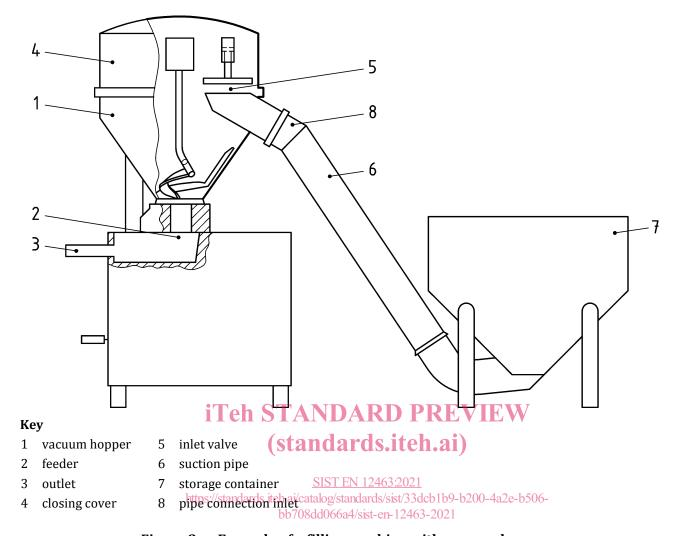
Figure 3 — Example of a filling machine with vacuum hopper
