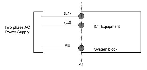
(L1, L2) Live AC terminals in 2 phases supply. PE Protective Earth.
