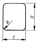
Figure — 8 mm Type S raw stock film
