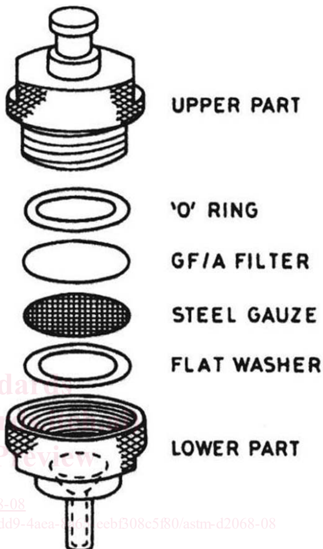
FIG. 1 Assembly of Filter A
