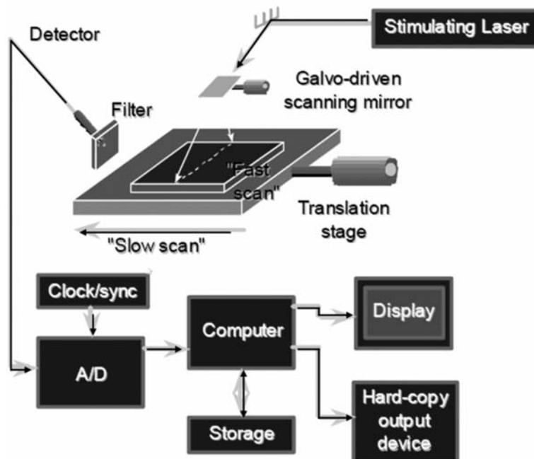
FIG. 4 Fundamental CR Image Acquisition and Display Process
