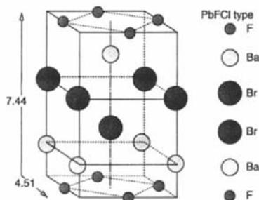
FIG. 8 BaFBr Crystal Structure
