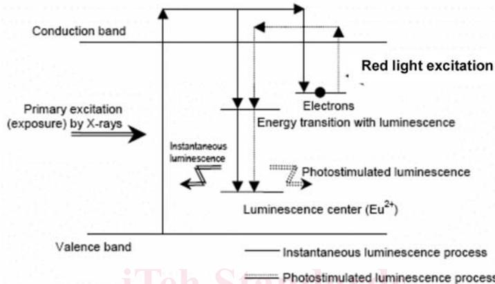
FIG. 10 Energy Level Diagram Illustrating Mechanism for Generating PSL in BaFBr: Eu<sup>2+</sup> Crystal
