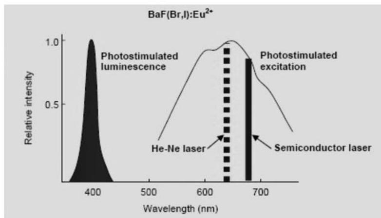
FIG. 7 Spectra of Photostimulated Luminescence and Excitation
