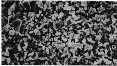
FIG. 9 Conventional BaFX: Eu Grains (10 microns)
