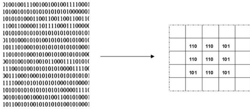
FIG. 5 Assignment of Binary Data to a Pixel Matrix (3 bit depth illustrated)
