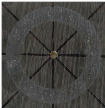
b) Correct test: Wear-through is not obtained in octants 4 and 5
