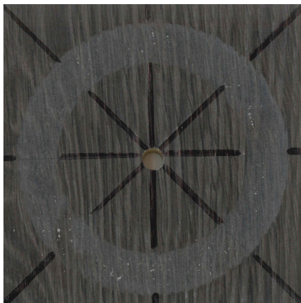
a) Insufficient test: Wear-through is evident only in one octant
