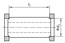
Figure 5 — Gauge-length measuring principle
